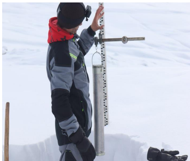
Digging out a snow sample (pit) to determine the drainage and snow density using a special industry tool in the Maykhura area in the Varzob River basin
